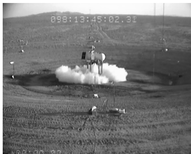
Fig. 2. Jack Rabbit chlorine release site, showing the 50 m diameter by 2 m deep depression and the tank set-up. This is the one-ton pilot release (Trial 2, see Table 1). The photo was taken about 2 s after the chlorine release began. Photo courtesy of Dugway Proving Ground.
