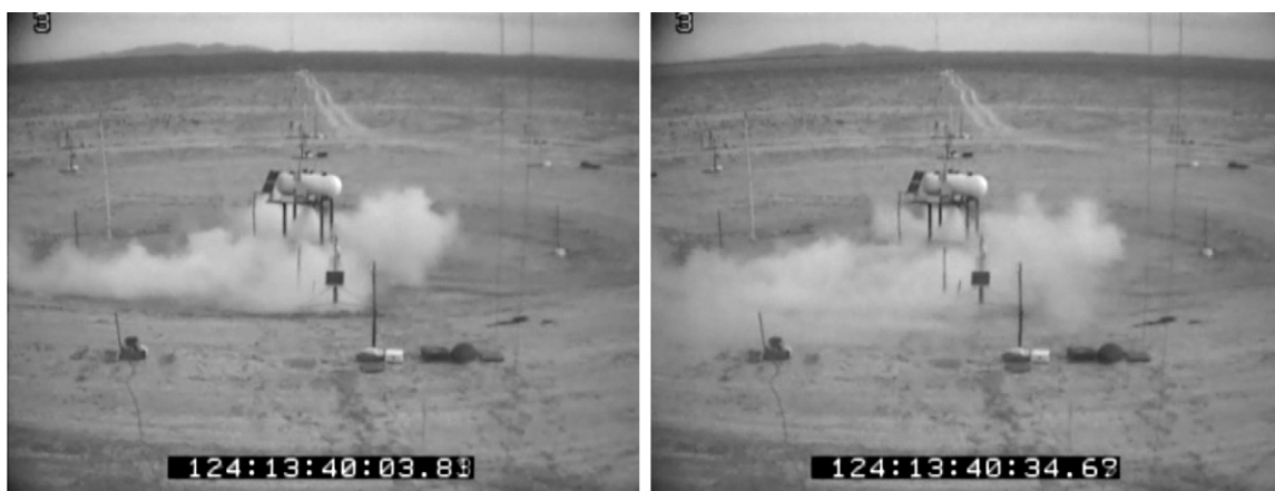
Fig. 4. Jack Rabbit Trial 6 (see Table 1) chlorine cloud, at 3 s (left), 34 s (center) and 180 s (right) after the release began. This is the high wind ( 6.2 \text{ m s}^{-1} ) trial. Photos courtesy of Dugway Proving Ground.
